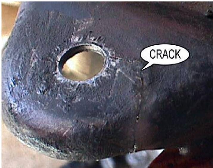
The crack in the control arm shown in the picture could have easily been found this way. This control arm was from an active GMC and had not yet failed. The GMCMM
